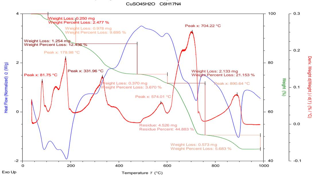
Figure 3. Derivatogram of the hexamethylenetetraammonium:copper sulfate system
