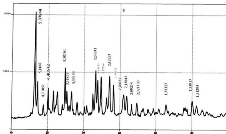
**Fig 2. X-ray pattern of hexamethylenetetrammonium:copper sulfate**
