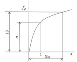
Figure 1. The dependence of the change in residual deformation  $f_c$  on the number of series (cycles) of deformation during experimental wear
