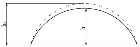
Figure 2. Evaluation of shape retention of tissue samples in a package according to conditional layouts in the form of a spherical segment
