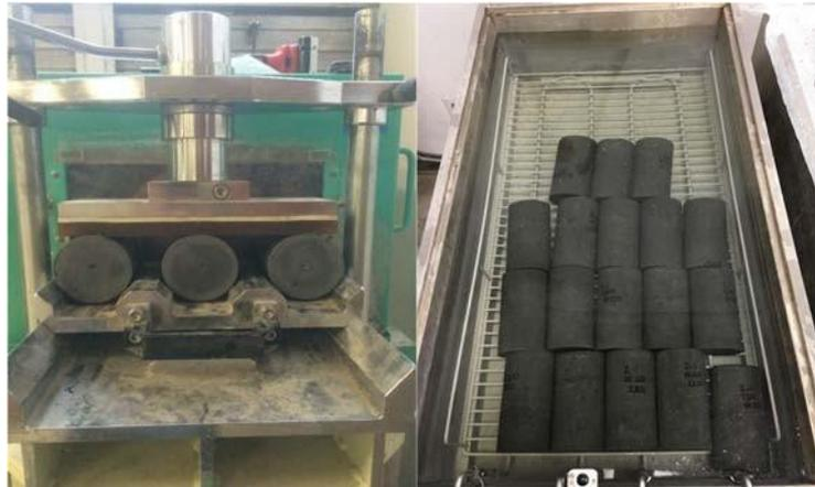
**Figure 3. End-grinder and water bath used for heat curing**
