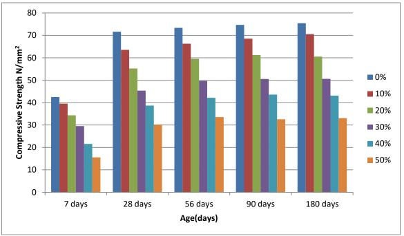
**GRAPH 3:** Variation of Compressive strength of <90 microns ceramic waste concrete mixes with age
