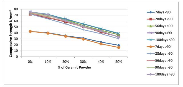
GRAPH 1: Compressive strength results of Ceramic waste powder concrete cured in normal water
