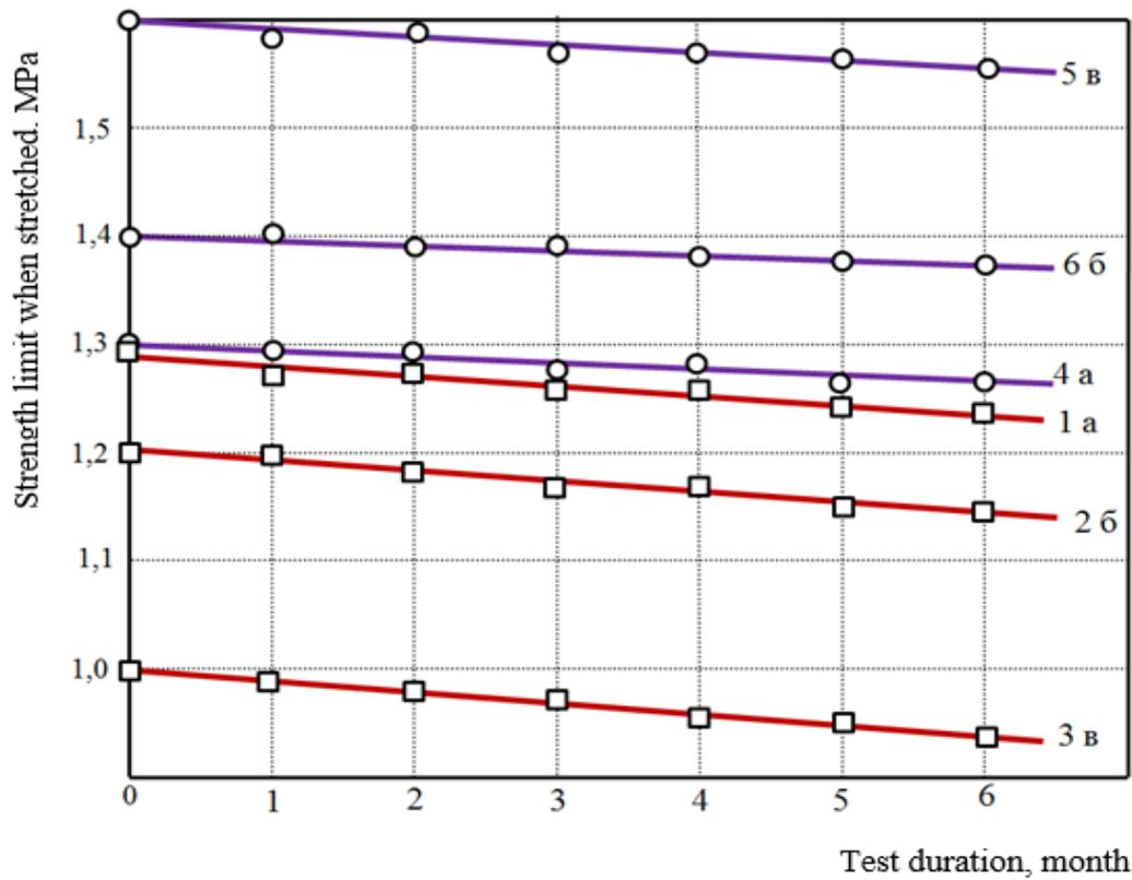
Fig. 1 Dependences of the tensile strength (1-6) of karakul skins over time on the consumption of formaldehyde (1-3) and glutaraldehyde (4-6), g / l: a-1, b-3 and c-5.
