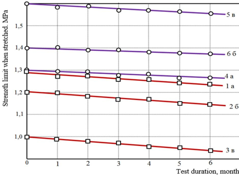
**Fig. 2 Dependences of the tensile strength (1-6) of astrakhan skins over time on the consumption of formaldehyde (1-3) and glutaraldehyde (4-6),g / l: a-1, b-3 and c-5.**
