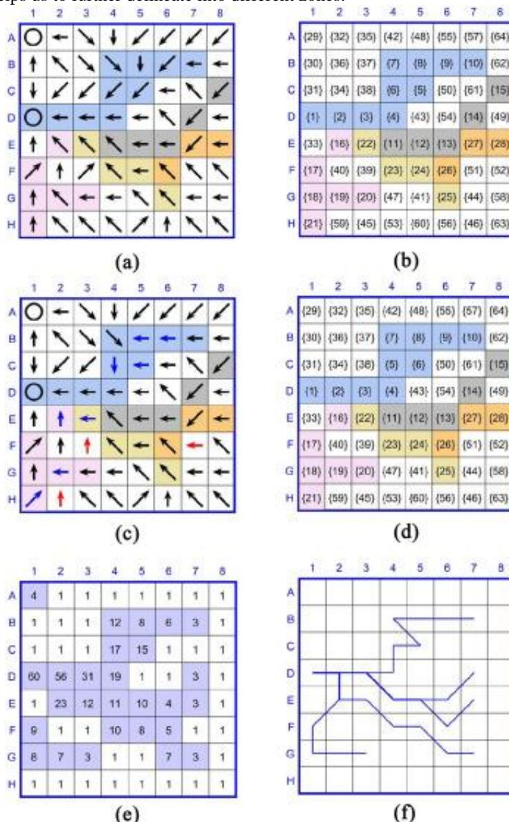
Fig 3. Digital numbers of DEM and ways of finding their path (Tao Wu et.al)
