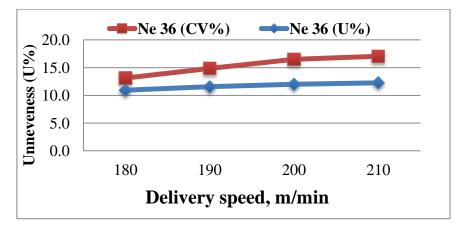
Pic. 1. Effect of the release rate on the uniformity of yarn, U % and CV % by Uster
