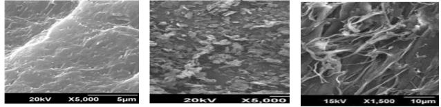
a) The structure of PEVP (outgoing, without filling); b) PEVP + kaolin AKS-30, 10 mass.ch + graphite 2.5 mass.ch; v) PEVP + kaolin (10) + graphite (2.25) + OShPP (4.0). Figure 3-Microstructure of heterocomposite materials on the basis of PEVP
