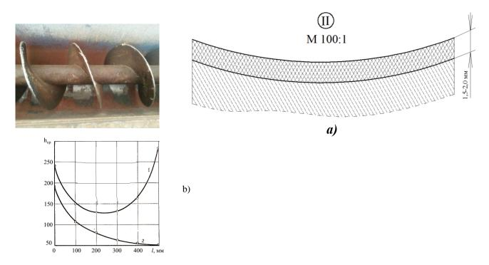
Figure 2. Scheme of obtaining multifunctional coatings containing GKP material -1,2,3 in cotton screw conveyor (distributor) screw and jellies (a) and their service life forecasting schedule (b).
