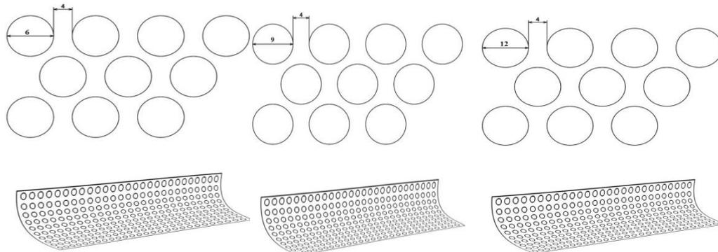
**Figure 1. Perforated fibre cleaning screens.**
