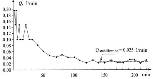
Fig. 2. An example of a graph of the dependence of water flow by ring on time according to the A.K. Boldyrev method
