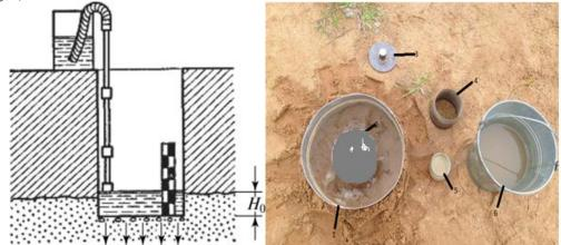
Fig. 1. Installation diagram for determination of filtration coefficient by A.K. Boldyrev method
