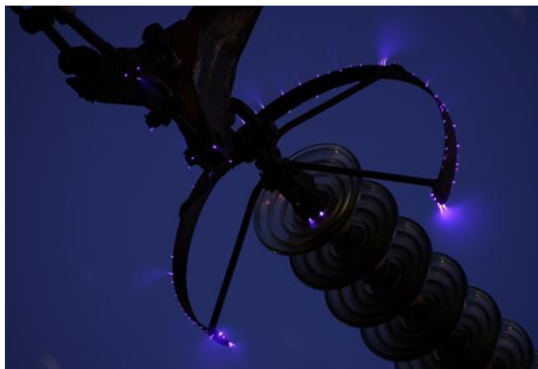
Figure 1. The image illustrates visible corona discharge occurring on a high-voltage overhead transmission line, primarily concentrated around the conductor surface, fittings, and insulator string.
