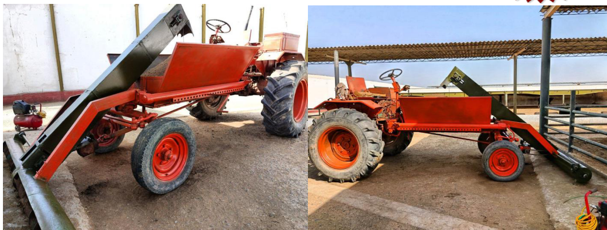
Fig. 1. General view of the mobile manure collection machine developed on the basis of a front-body tractor
