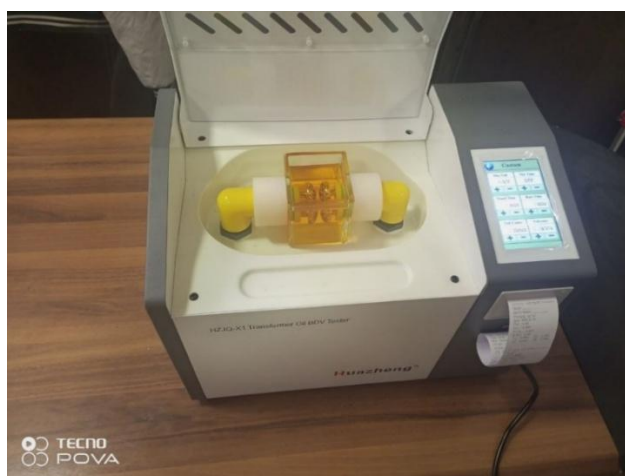
Fig 1. HZJQ-X1 device measuring transformer oil electrical strength
