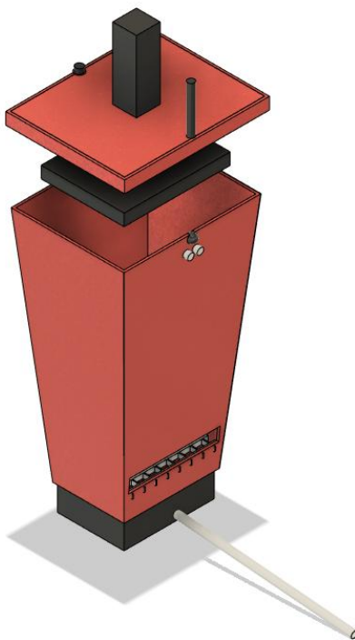
Figure 2: Isometric Layout of the Automated Waste Management Unit
