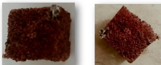
Fig.2. PUF modification ( \text{rGO}/\text{Fe}_3\text{O}_4/\text{PUF}/\text{PS} ).
