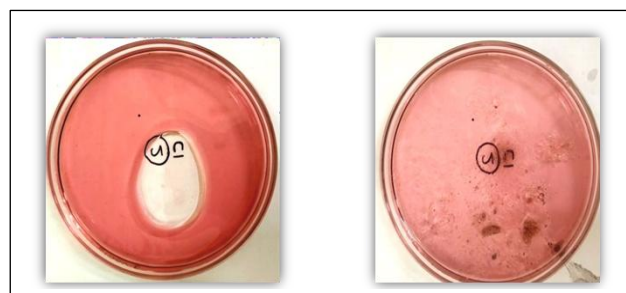
Fig.4. Absorption of chloroform from water with rGO/ \text{Fe}_3\text{O}_4 /PUF/PS.
