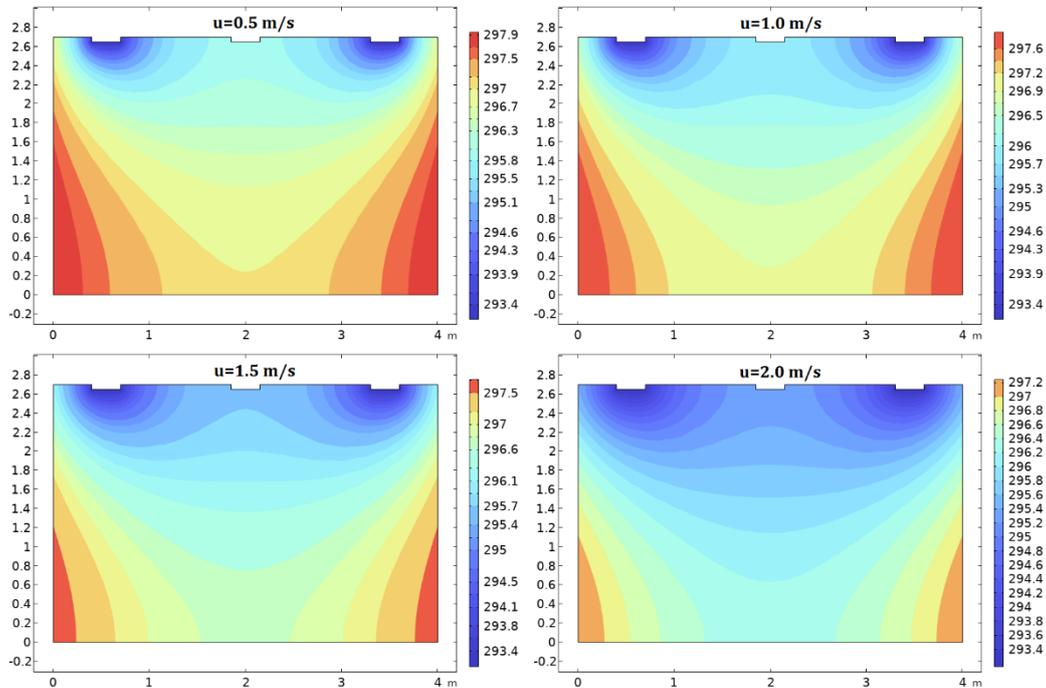
**Figure 4. Temperature field for indoor air in the experimental house**
