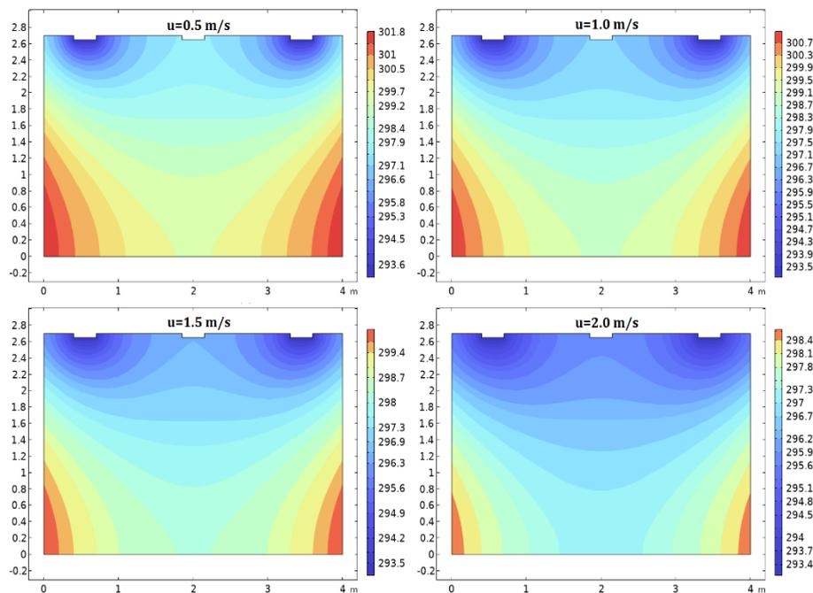
Figure 6. Temperature field for indoor air in the experimental house
