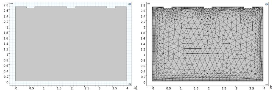
**Figure 2. 2D model of an experimental house with an air-cooled system (a) and computational mesh (b)**
