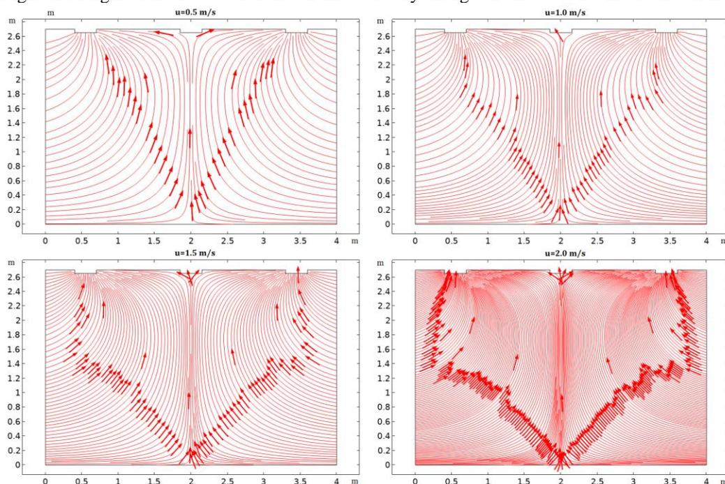
**Figure 3. Convective heat flow characteristics in the experimental house**
