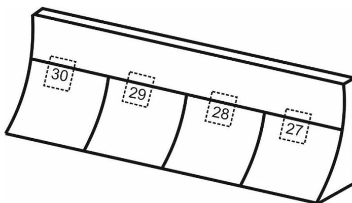
Figure 2. Bulldozer blade with four vibration exciters.
