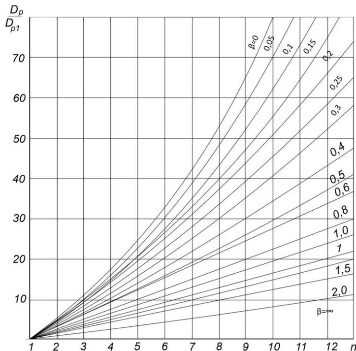
Figure 1. Nomogram for determining the  $\beta$  parameter.
