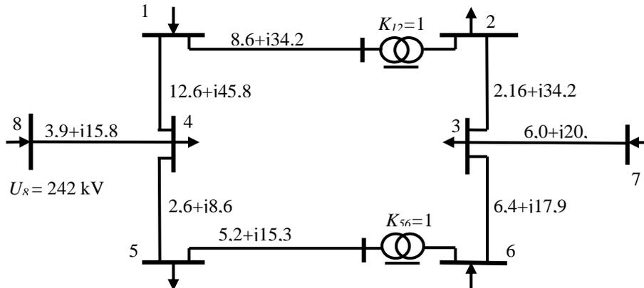
Fig. 1. Electrical network diagram of EPS.
