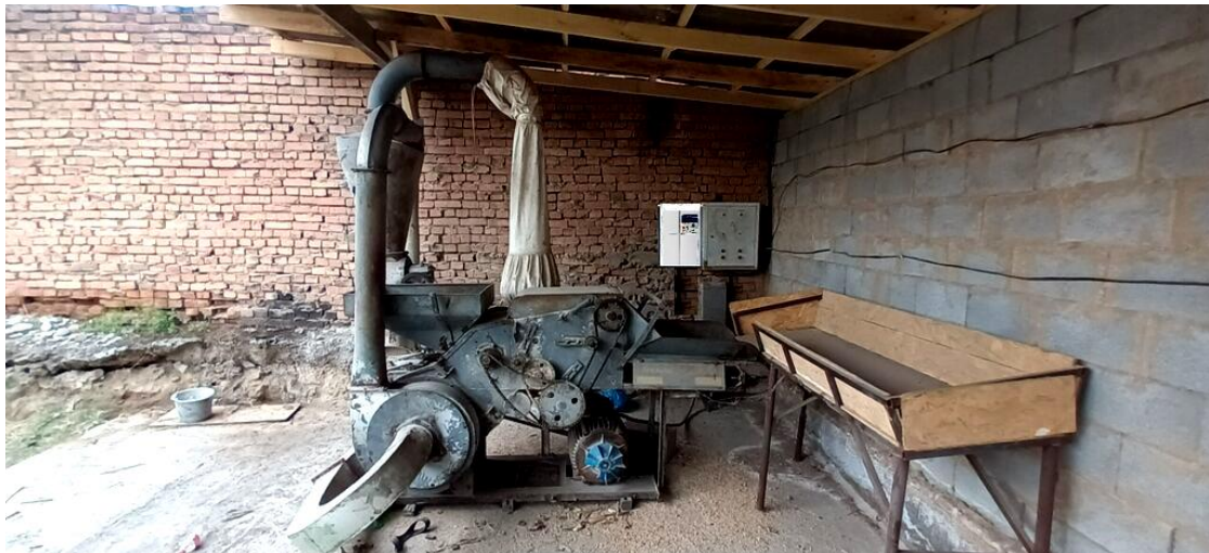
Fig. 1. General view of controlling an asynchronous motor of a universal fodder shredder using a frequency converter
