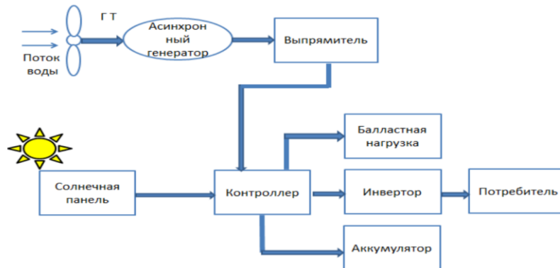
Fig. 2. Block diagram of the device transfer to the load via the controller [6].
