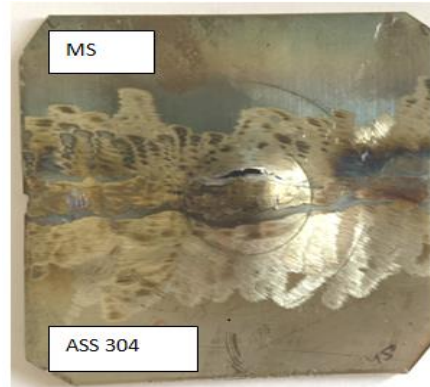
Fig.3.1 Deformed sheet metal butt weld specimen from Erichsen cupping test
