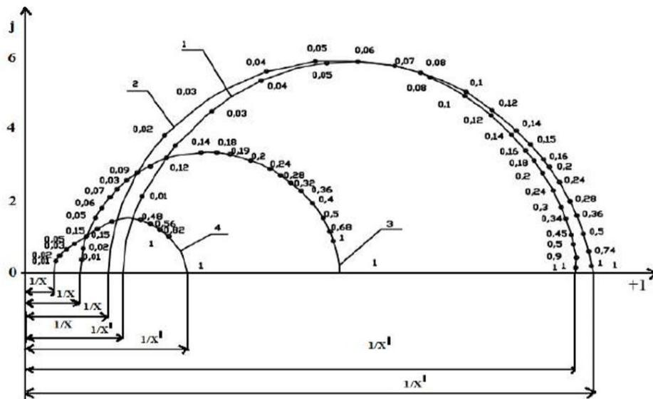
Fig. 3. Frequency responses of model asynchronous Turbogenerators, where: 1 - massive rotor with short-circuited copper cages,  $Z_2=80$ ; 2 - massive rotor with short-circuited copper cages,  $Z_2=48$ ; 3 - massive toothed rotor; 4 - massive smooth rotor.
