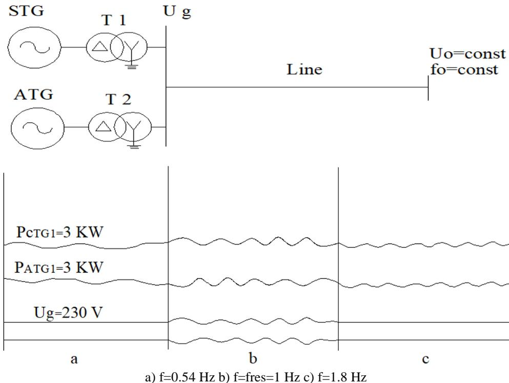
Fig.1. Oscillograms of periodic power fluctuations of SG and AG.
