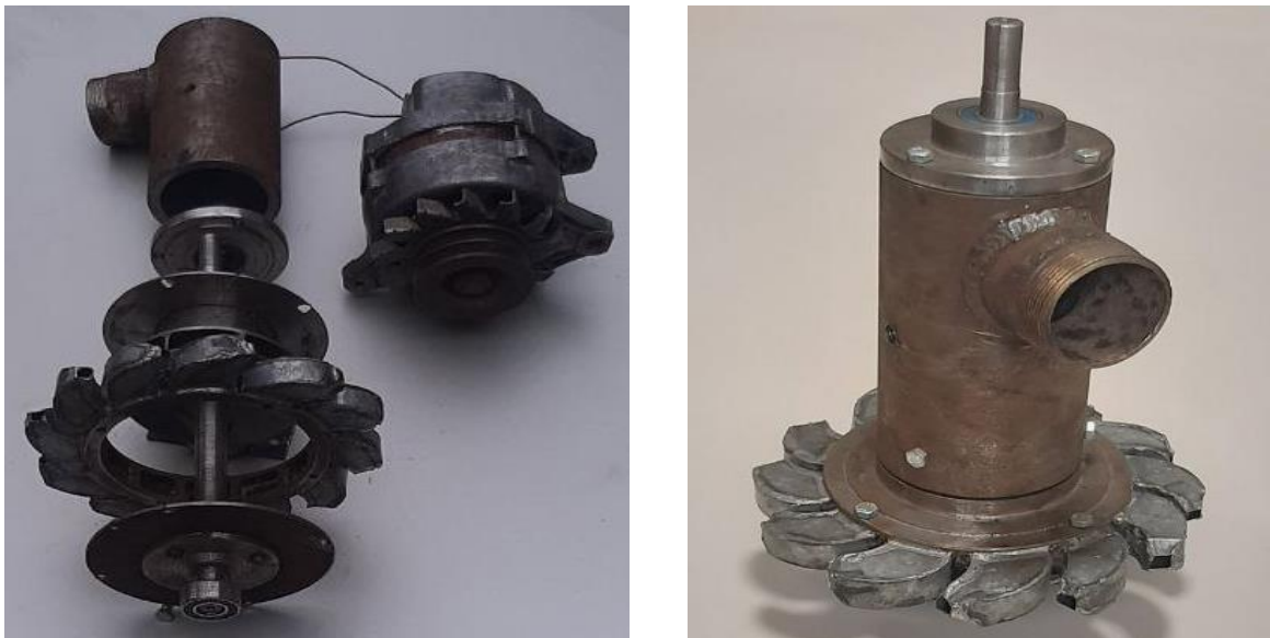
Fig. 2. An experimental model of a pico hydro turbine with an internal guiding device.
