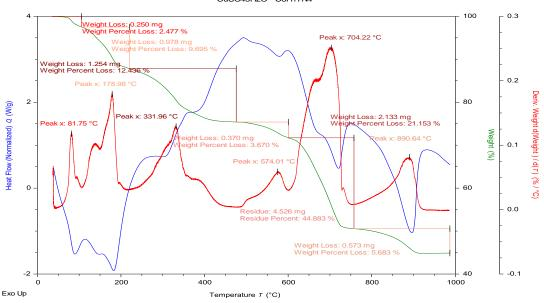
Figure 3.Derivatogram of the hexamethylenetetraammonium:copper sulfate system
