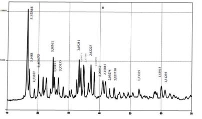
Fig 2. X-ray pattern of hexamethylenetetrammonium:copper sulfate
