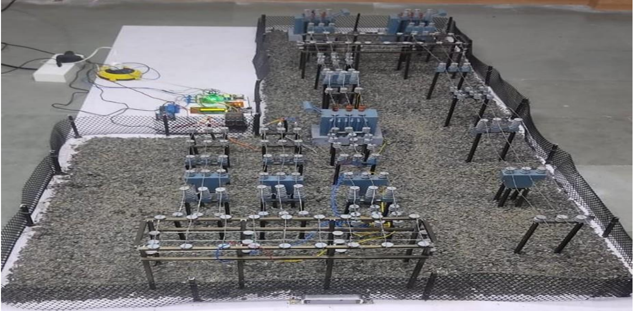
Fig. 6.1 Miniature Working Model of 33/11 kV Substation
