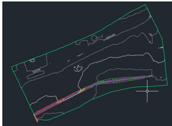
Fig.1: Horizontal Alignment generated by AutoCAD Civil 3D
