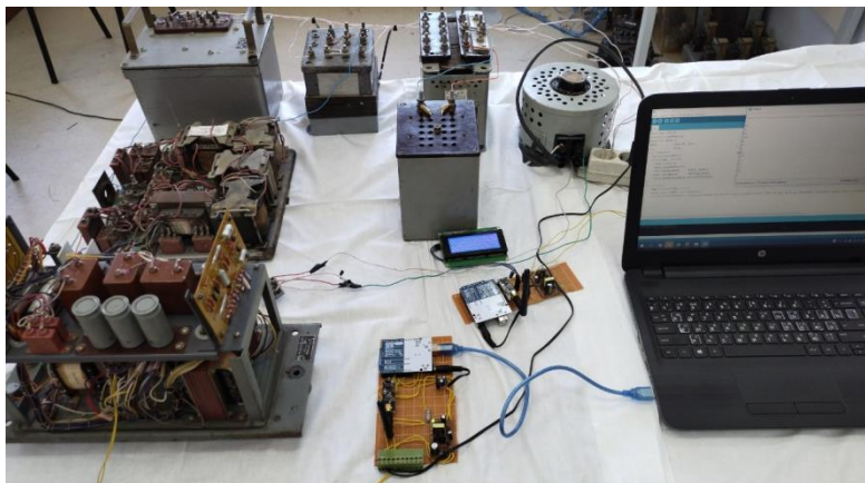
Figure 5. The appearance of the automatic locomotive signaling signal control device in the laboratory
