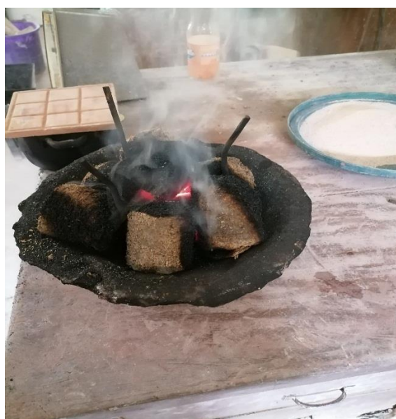
Plate 2: Combustion performance test of the briquettes – torrefacted briquettes on the left and non-torrefacted briquettes on the right.
