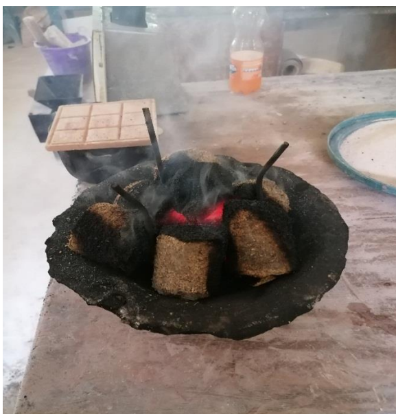
Plate 2: Combustion performance test of the briquettes – torrefacted briquettes on the left and non-torrefacted briquettes on the right.
