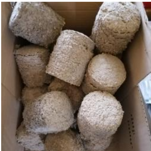
Plate 1. The extruded biomass briquettes after drying. Notice the color difference between the non-torrefacted batch on the left and the torrefacted batch on the right.
