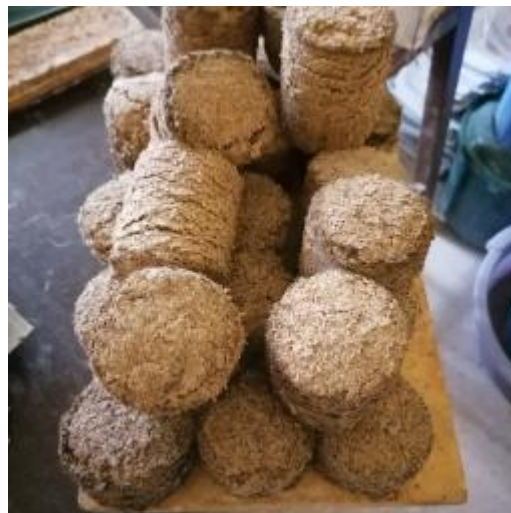
Plate 1. The extruded biomass briquettes after drying. Notice the color difference between the non-torrefacted batch on the left and the torrefacted batch on the right.
