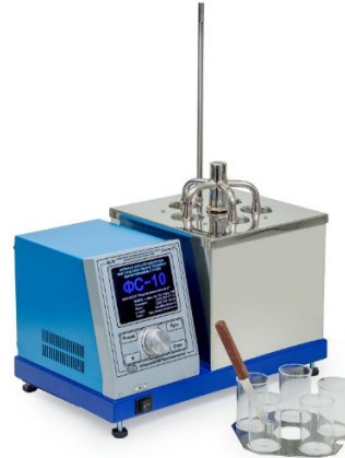
Picture. The device for determining the amount of tars FS-10
