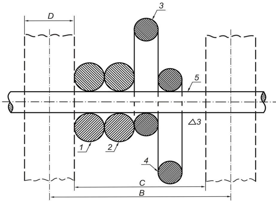
Figure 2, Schematic of the formation of terry fabrics, cross-section of pile and ground warp yarns.
