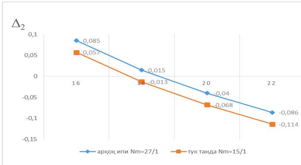
Figure 5. The distances between the pile warp and the weft yarns.
