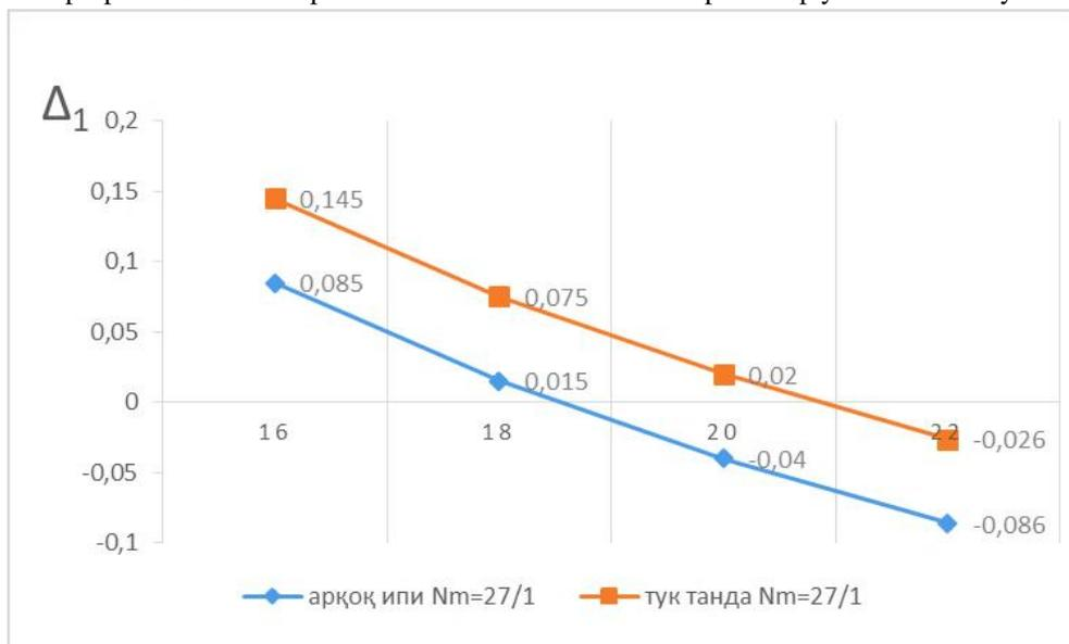
Figure 4. The distances between the ground warp and the weft yarns.
