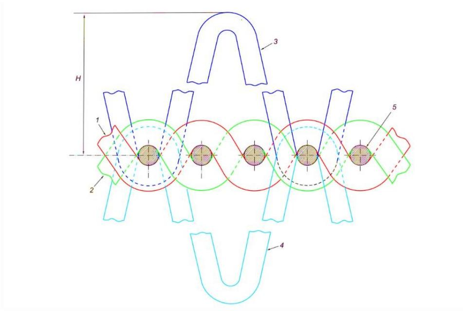
Figure 1, Scheme of formation of terry fabrics, section cut the weft yarn.
