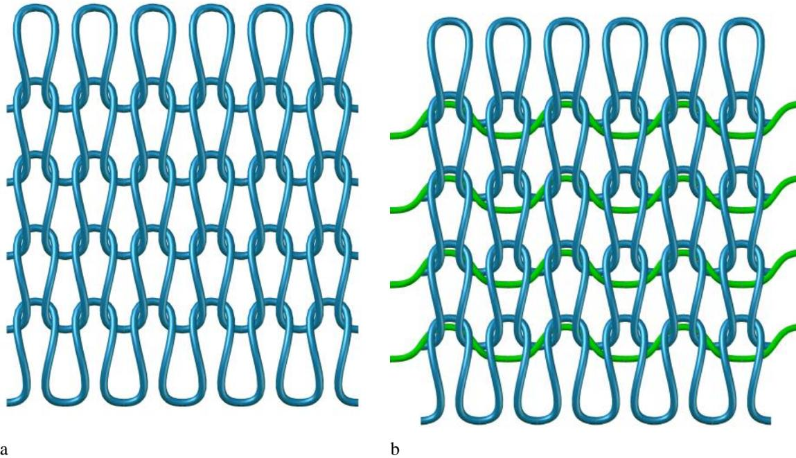
Fig1. Knitting structures for using in medicine a) plain structure b) fleecy structure
