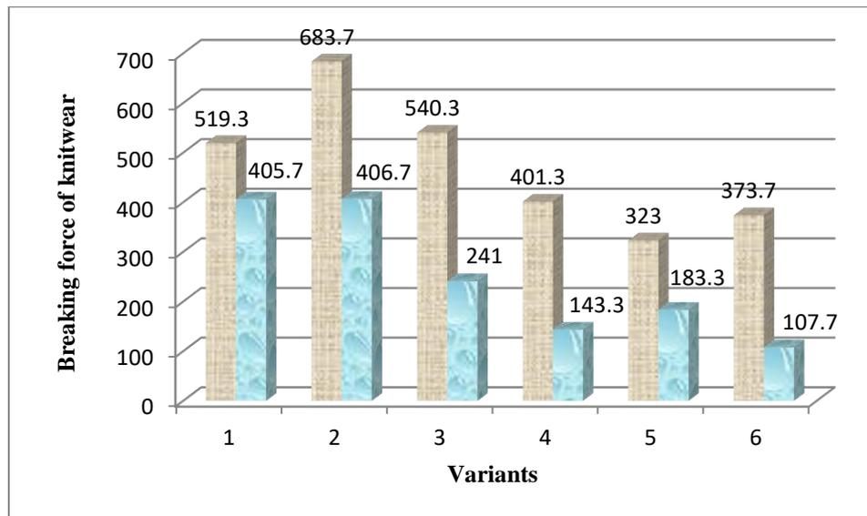
Fig4. Histogram of changes in the breaking force of knitwear for using in medicine
