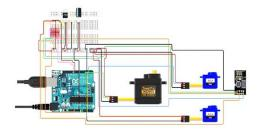
Fig no. 4 Arm circuit diagram
