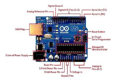
Fig No. 5 Arduino UnoR3 board [9]
