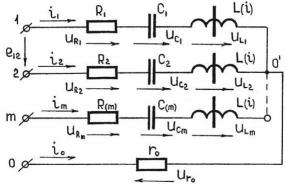
Figure 1. Multiphase ferroresonant circuit with zero conductor and no ferromagnetic coupling between the non-linear coils.
