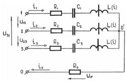
Figure 2. Three-phase ferroresonant circuit with symmetrical power supply.
