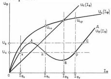
Figure 3. Voltammetry characteristic of one phase of a three-phase ferroresonant circuit.
