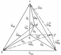
Figure 4. Topographical diagram of the phase and line voltages of a three-phase unbalanced ferroresonant circuit (at fundamental harmonic).
