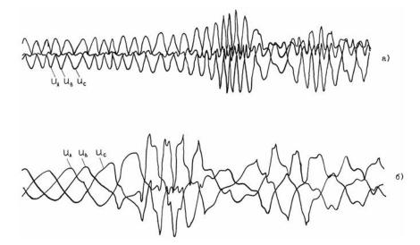
Fig.2. Oscillograms of phase voltages of a three-phase circuit with separate (a) and common (b) magnets in auto parametric oscillation excitation mode.
