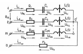
Figure 3. Multi-phase ferroresonant circuit with zero conductor and no ferro-magnetic coupling between the non-linear coils.
