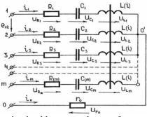
Figure 5.Multi-phase ferroresonant circuit with zero conductor c ferromagnetic coupling between the non-linear
