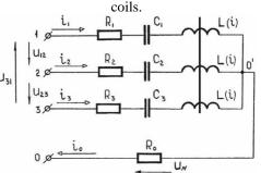
Figure 6.Three-phase ferroresonant circuit with zero-wire c ferromagnetic coupling between the non-linear coils.
