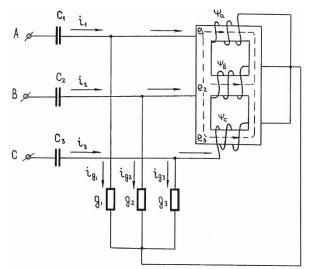
Figure 1. Three-phase ferroresonant AP circuit with magnetic coupling between phases without a neutral conductor.
