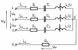
Figure 4. Three-phase ferroresonant circuit with symmetrical power supply.
