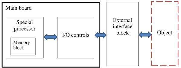
Figure 3. The generalized structure of the hardware-software platform.
