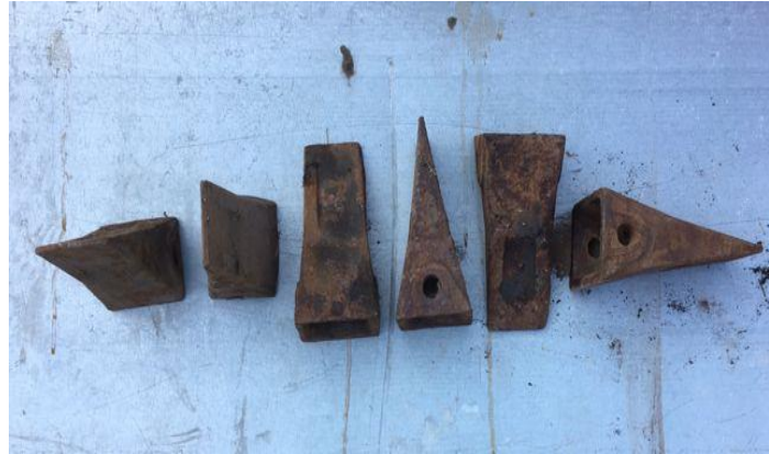
Defective parts with non-metallic inclusions and holes.
