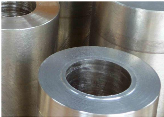
Detailed image of the sand-clay mold according to the results of the research. After machining.
