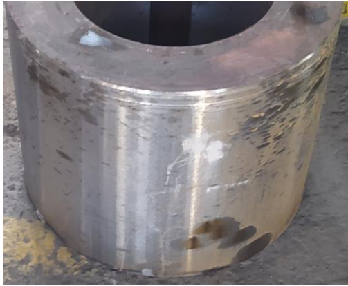
Defective parts with non-metallic inclusions and holes.
