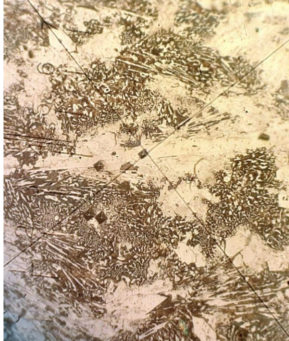
Fig. 5. Measurement of microhardness of primary cementite
