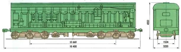
Figure: 1. Weight-checking wagon of 640-VPV type
