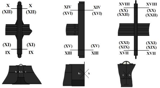
Figure: 4. Scheme for measuring the thickness of sheet wear on the pivot beam of the weighing wagon frame
