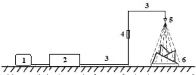
Figure 3. Schematic of the laboratory device: 1 - capacity; 2 - pump; 3 - pipe; 4 - water meter; 5 - sprayer; 6 - Fireplace Upon completion of the experiment, the mean values of the 3 experiments performed with each suspension and water were entered in Table 4 and a comparative graph (Figure 4) was prepared based on it.
