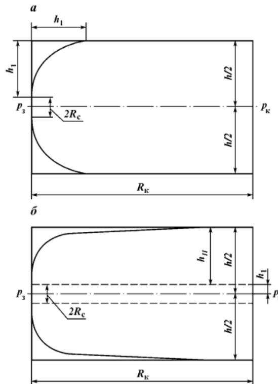
**Fig. 4. Scheme of gas inflow to a horizontal well: a - with a parabolic nature of the change in  $h(R)$  in the bottomhole zone; b - with a hyperbolic nature of the change in  $h(R)$**
