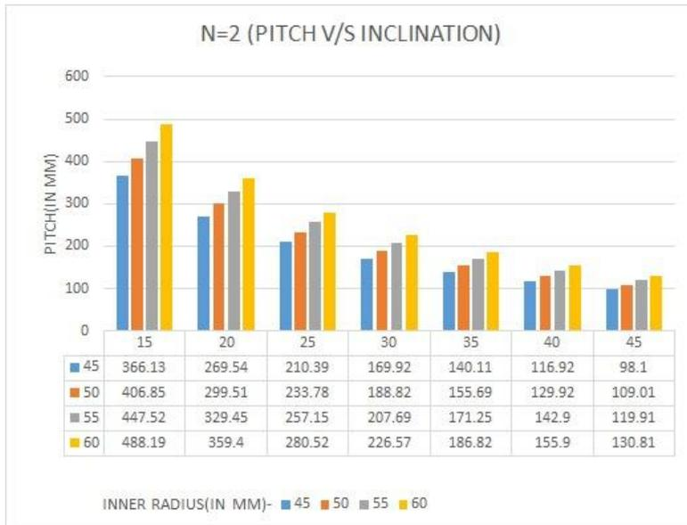
The graph shows the representation of Pitch vs Inclination for a screw start of 2 (N=2). The different colours represent inner radii. The graph shows that the pitch decreases with increase in angle of inclination.
