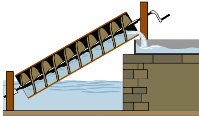
Fig 1.1 Archimedes Screw Pump<sub>[1]</sub>
