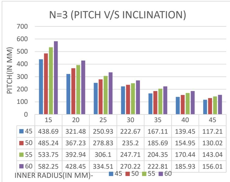
The graph is the representation of Pitch vs Inclination for a screw start of 3 (N=3). The colours show different lengths of inner radii of the helical screw. From the graph, we can observe that the pitch decreases with increase in angle of inclination.
