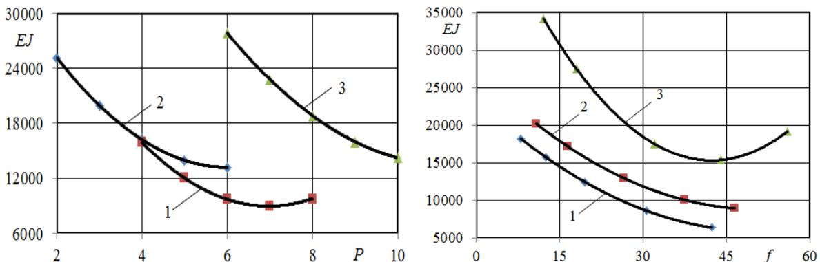
**Fig. 3. Dependences of stiffness  $EJ$  on the value of the bend force  $P(a)$  and the value of the bend  $f(b)$  for different diameters of corn stalks:**
