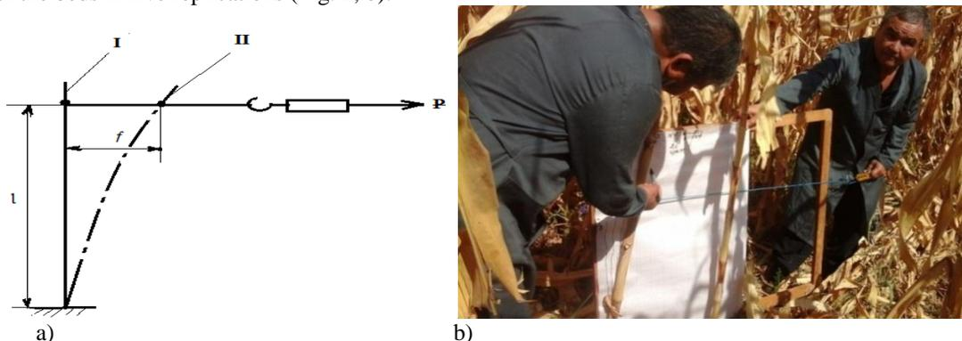
**Fig. 2. Scheme for defining the limb of stems (a) and a fragment of the type of field experiments (b):** I-initial position of the stem; II-position of the bend of the stem after the application of force;  $l$ -height of the bend force setting;  $P$ -bending force;  $f$ -bend amount
