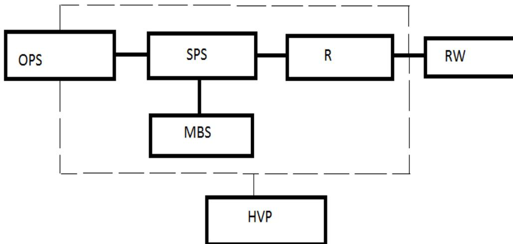
**Fig. 1. The principle of operation of the quantum generator: OPS - optoelectronic power supply; SPS - sorting focusing system; MBS- molecular beam source; P - resonator; RW- radiated waves; HVP- high vacuum pump**
