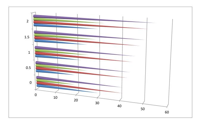
In general"Betonstrong17"we determined the compressive strength when we added the superplasticizer PTs-400 D20 in Portland cement at 0.5-1-1.5-2%, and when we added the optimal amount of 2% to 37 MPa under normal conditions for 7 days, and after 28 days At 48 MPa, -5 °C, it reached 35 MPa in 7 days and 44 MPa in 28 days.
