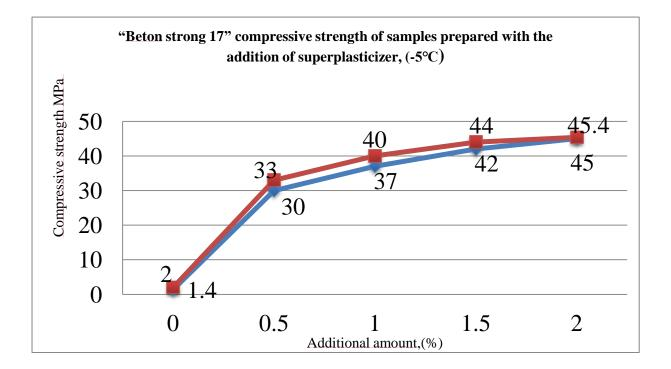
In general "Beton strong 17" We determined the compressive strength of the superplasticizer PTs-400 D20 in Portland cement at 0.5-1-1.5-2%, and the optimal amount of 2% at -5 °C at 45 MPa for 7 days and 28 days. then reached a strength of 45.4 MPa.
