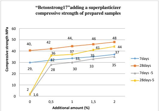
The following table shows the compressive strength of concrete prepared by reducing the S / S ratio.
