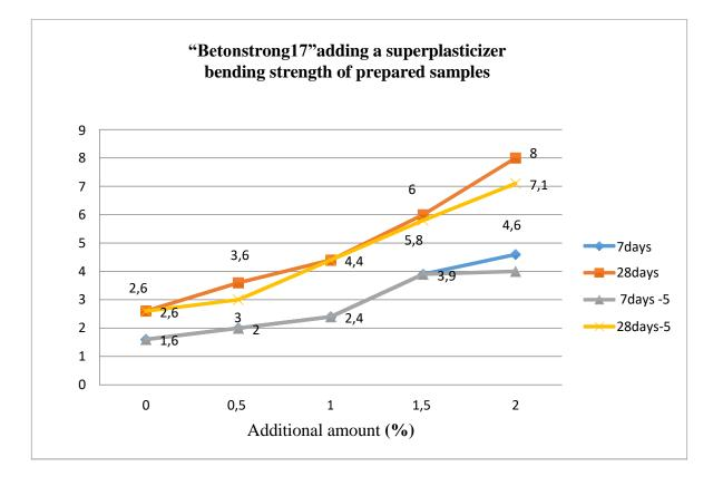
The following table shows the results of bending strength with reduced water content
