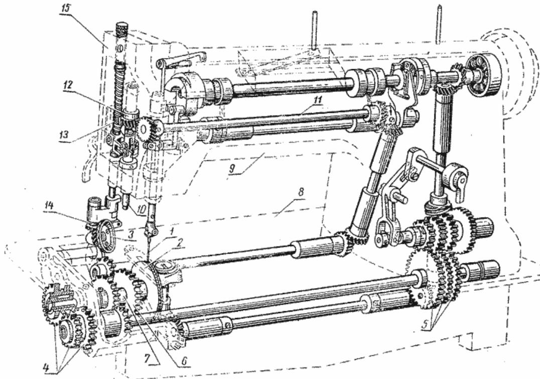
**Fig. 1. Kinematic diagram of a sewing machine.**
