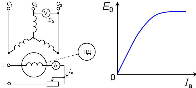
Fig. 5. Idling characteristic of the synchronous generator G-273A
