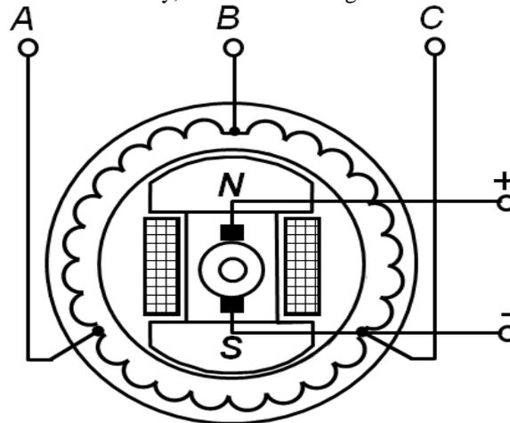
**Figure 1. Scheme of a synchronous machine.**
