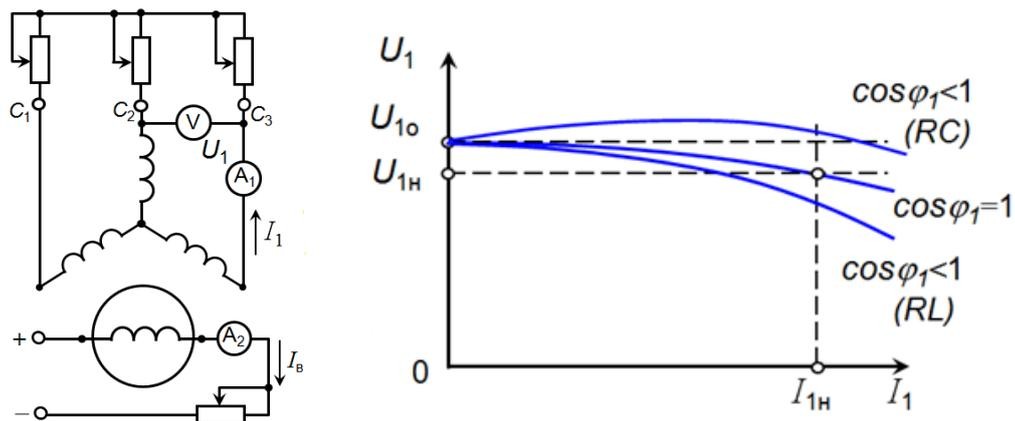
Fig. 6. External characteristic of the synchronous generator G-273A.
