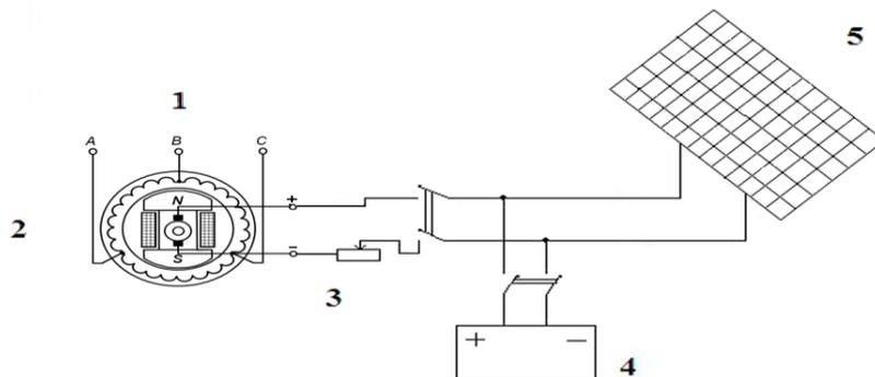
Fig. 4. Excitations of synchronous machines by a solar battery.
