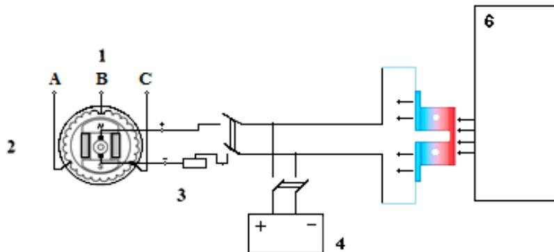
Fig. 2. Excitation of synchronous machines by a thermoelectric generator
