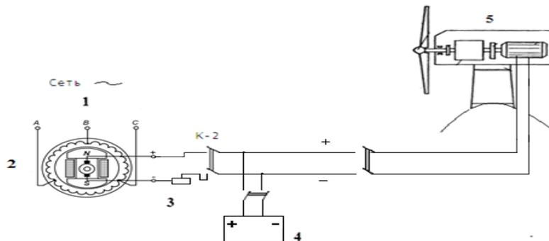
Fig. 3. Excitation of synchronous machines from a solar battery.
