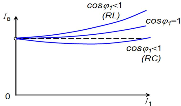
Fig. 7. Adjustment characteristic of the G-273A synchronous generator.
