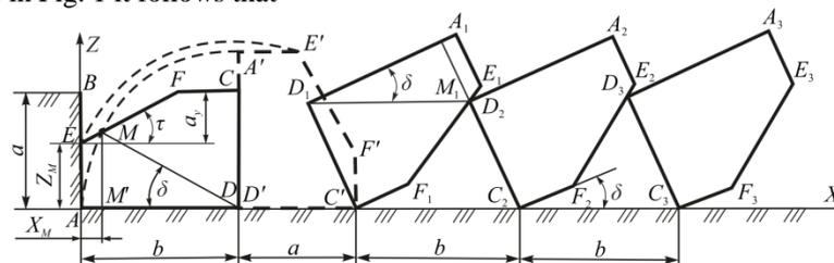
Fig. 1. Scheme for studying the process of formation rotation by a housing with an angle-removable housing and determining the angle of inclination of the dumped formation to the bottom of the furrow
