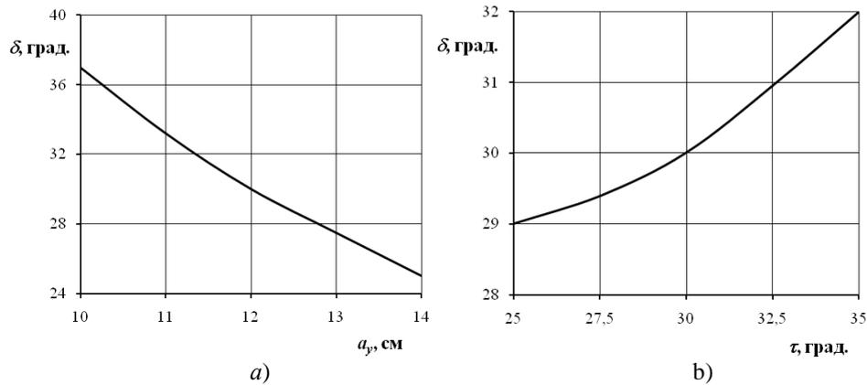
Fig. 2. The dependence of the angle of inclination of the dumped formation to the bottom of the furrow from  $a_y$  (a) and  $\tau$  (b)
