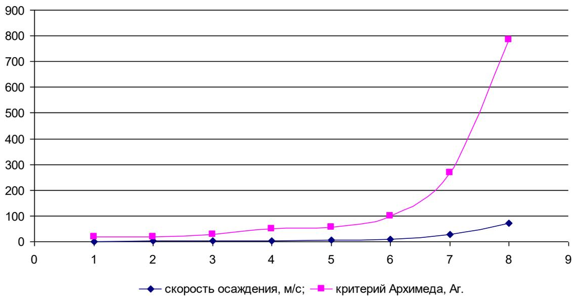
Fig.2. Change the criterion of the Archimedes depending on the rate of precipitation of solids in the centrifugal field
