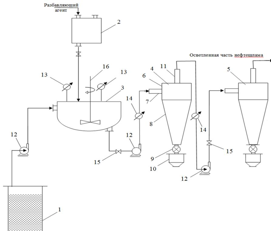
Fig. 1. Purification of oil sludge from mechanical impurities: 1- capacity for oil sludge supply; 2- capacity for supplying a diluting agent; 3,16-capacity with a stirrer; 4,5-hydrocyclones; 6- cylindrical part of the hydrocyclone; 7 - a supply pipe of a hydrocyclone; 8 - conical part; 9- lock gate; 10- hopper for trapped mass; 11 - drain pipe; 12 - pumps; 13- manometers and thermometers; 14- flowmeters; 15 - gate valves.
