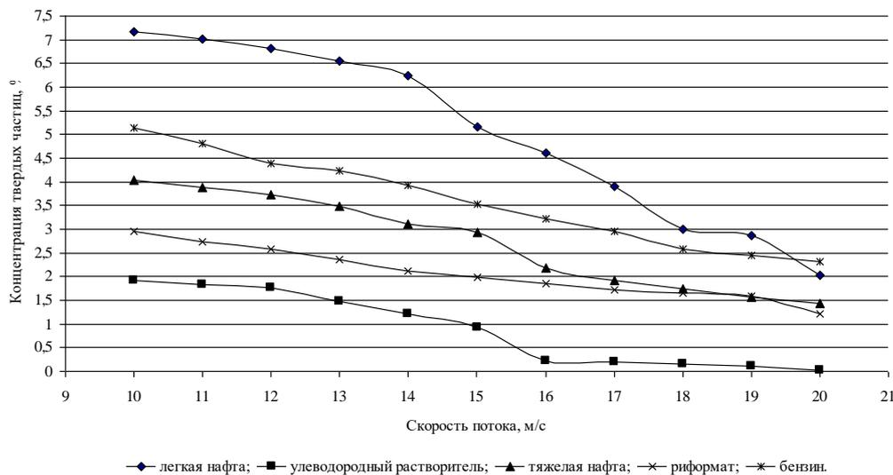
Fig.2. The change in the residual concentration of solid particles depending on the flow rate.
