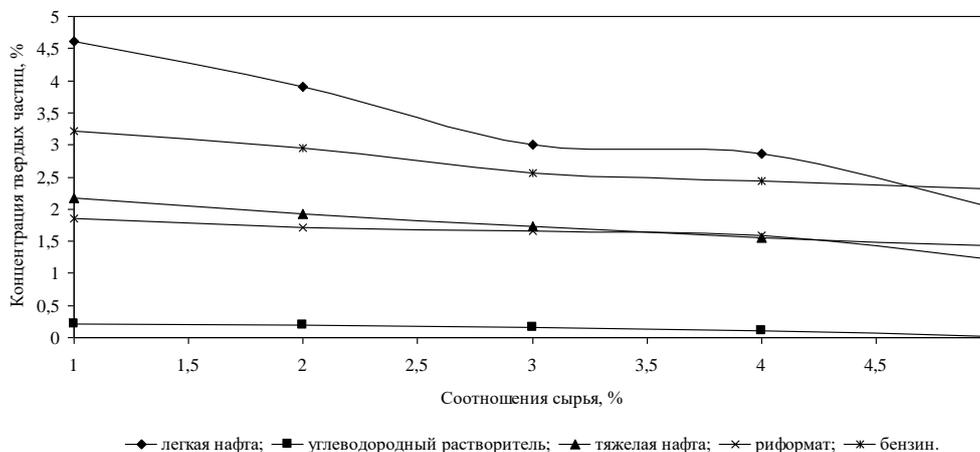
Fig.3. Changing the concentration of solid particles in the composition of the oil sludge, depending on the ratio of the solvent
