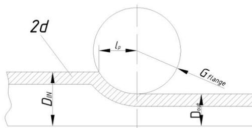
Fig. 5. Caliber seam crimping unit
