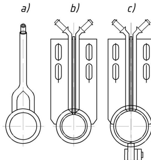
Fig. 2. Designs of inductors for welding longitudinal pipes:
