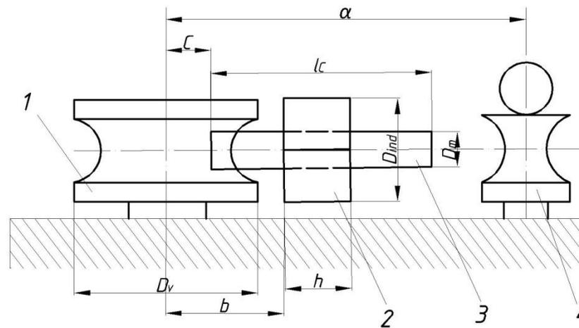
Fig. 1. The scheme of the welding machine of the mill of high-frequency welding of longitudinal pipes:
