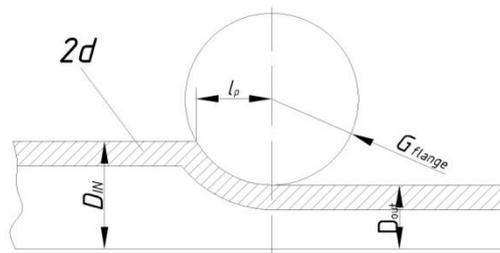
Fig. 5. Caliber seam crimping unit
