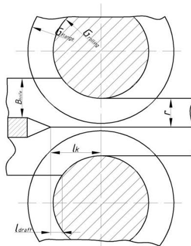
Fig. 4. Diagram of upsetting edges when welding a pipe billet of radius  $r$ :
